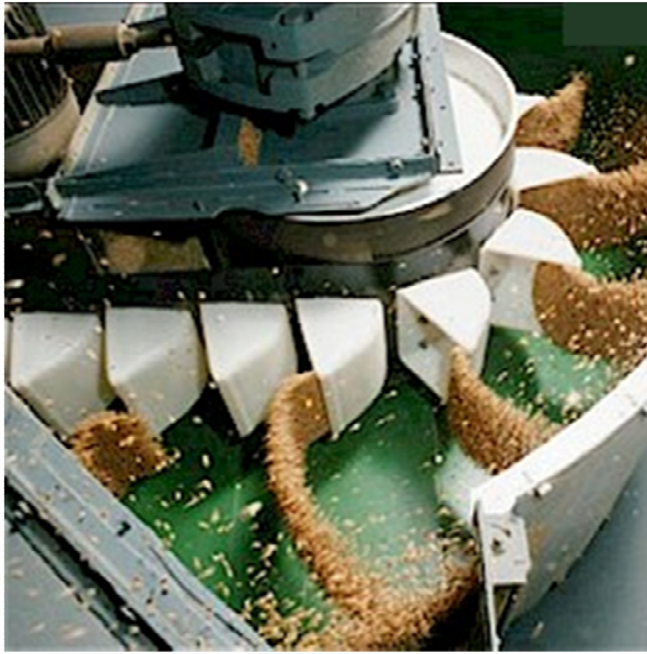
Figure 3.2 Unloading section of chain bucket elevator
